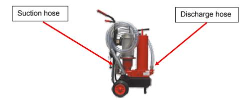
During operation the open end of the suction line has to be minimum 100 mm below the fluids surface. Also, make sure that the fluid circulation is not blocked at both ends of the hoses. Please use the pipe connections included in delivery, if the hoses will be connected to any pipe work. The filter unit is switched on and off at the combined OFF-ON and motor protection switch.
