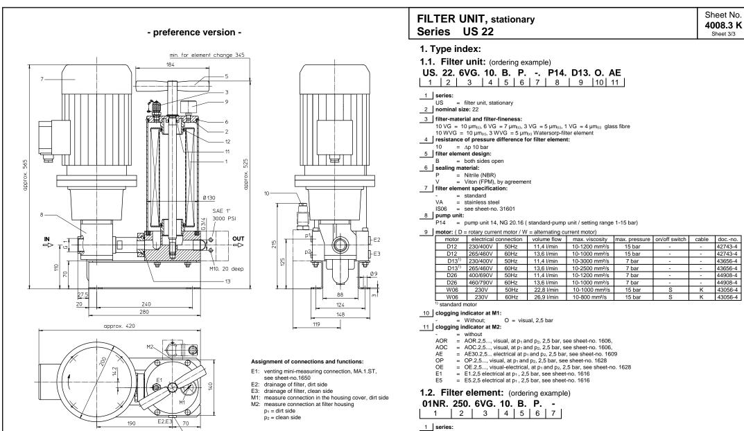
01NR. = standard-return-line filter element according to DIN 24550, T4
