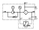
Filter unit with visual clogging indicator AOR. AOC. OP
