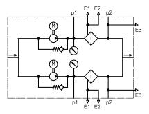
Filter unit with electrical clogging indicator AE30
