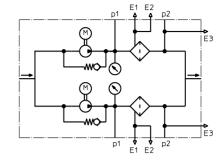
Filter unit with electrical clogging indicator AE30
