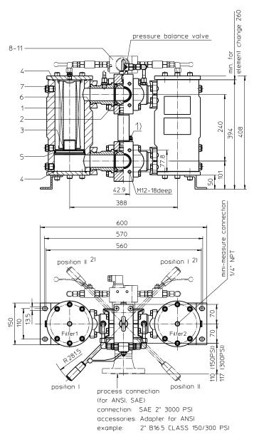
Position I: Filter 1 in operation Position II: Filter 2 in operation
