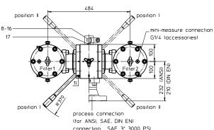
1) Connection for the potential equalisation at inlet and outlet, only for application in the explosive area.
