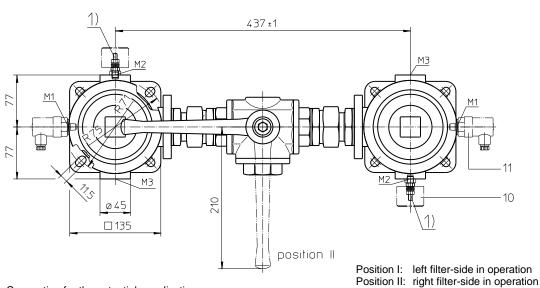
Connection for the potential equalization, only for application in the explosive area.
