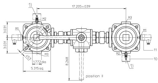
Position I: left filter-side in operation Position II: right filter-side in operation
