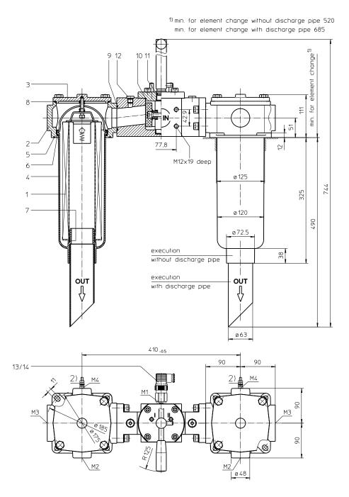
2) Connection for the potential equalization, only for application in the explosive area.
