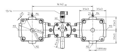
$^{(1)}$  min, for element change without discharge pipe 20.47 min, for element change with discharge pipe 26.97
