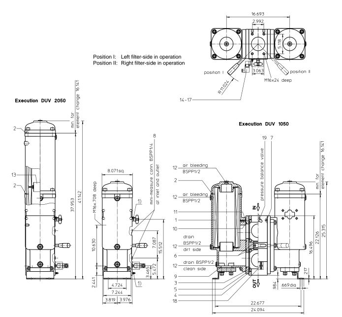
1) Connection for the potential equalization, only for application in the explosive area.
