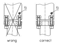
1) Connection for the potential equalization, only for application in the explosive area.
