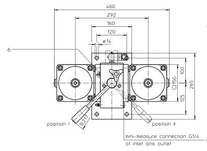
Connection for the potential equalization, only for application in the explosive area.
