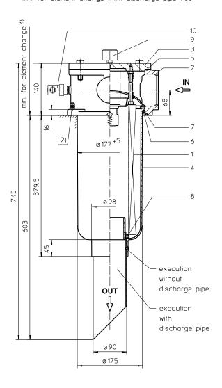
2) Connection for the potential equalization only for application in the explosive area.
