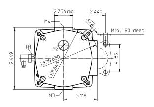
1) min. for element change without discharge pipe 22.04 min. for element change witht discharge pipe 30.70
