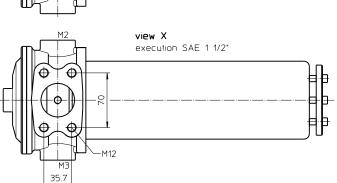
1) The bypass valve is integrated in the screw plug. For the filter without a by-pass valve the opening function is raised up to  $\Delta p > 1$  bar
